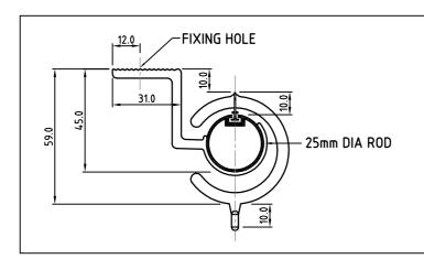
Ceiling to top of rod: 20mm
