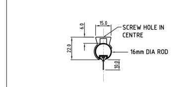
Ceiling to top of rod : 6mm Ceiling to bottom of rod : 22mm Glide sits 10mm below rod
