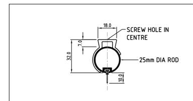
Ceiling to top of rod : 7mm Ceiling to bottom of rod : 32mm Glide sits 10mm below rod
